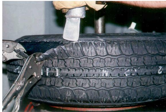
Figure 3. Tire Prep for Tread Separation Simulation.
