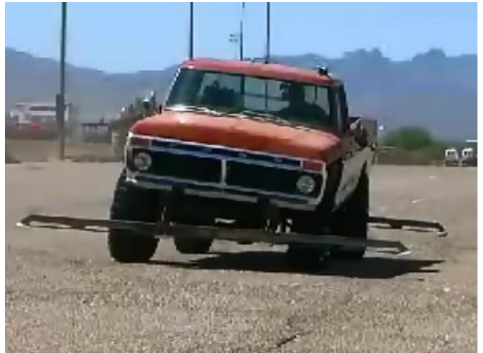
Photo 6. Significant lean of the truck after the left front tire was flat.
