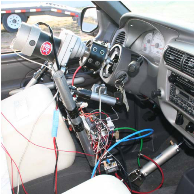
Figure 1. Remote-controlled steering and braking system.
