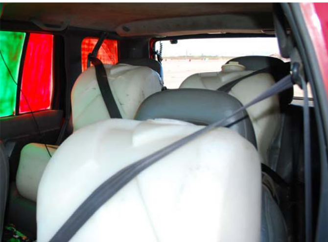
Figure 4. Salt-filled dummies in vehicle seating positions for Test 4.
