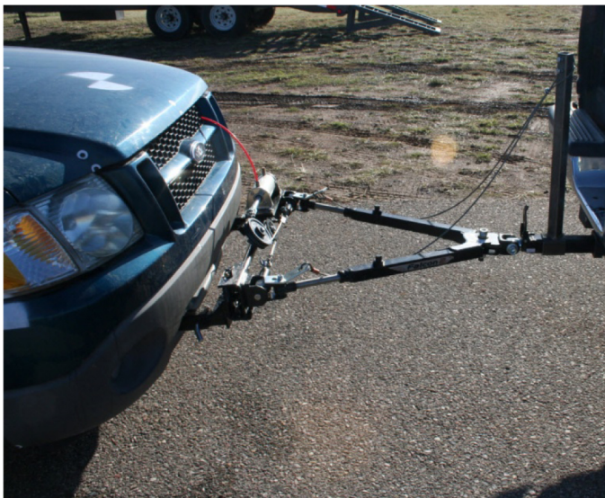
Figure 2. Towing and pneumatic release system for Test 2.
