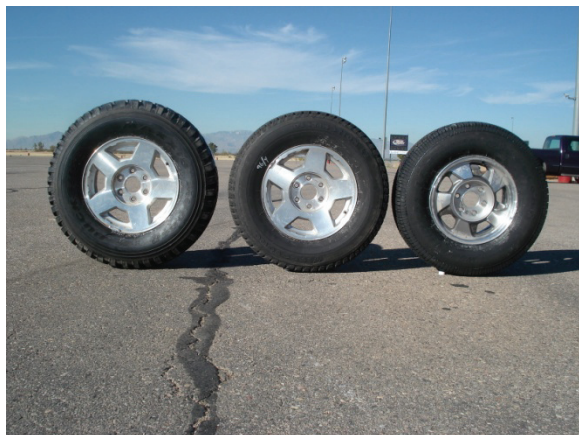
Photograph 3. From left to right: (3) Buckshot Maxxis Mudder LT285/70R17; (1) Firestone Destination LE P265/70R17; (2) Firestone Wilderness LE P265/70R16.
