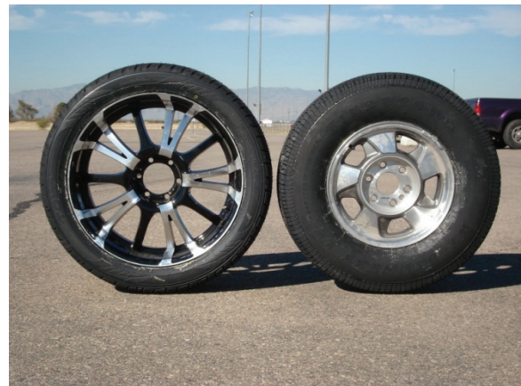
Photograph 5. From left to right: (4) Toyo Proxes S/T P305/40R22 and (2) Firestone Wilderness LE P265/70R16.
