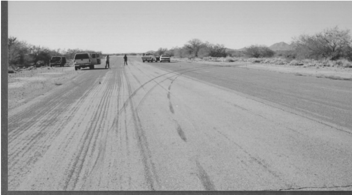
Photograph 3. Hopping rear tire marks
