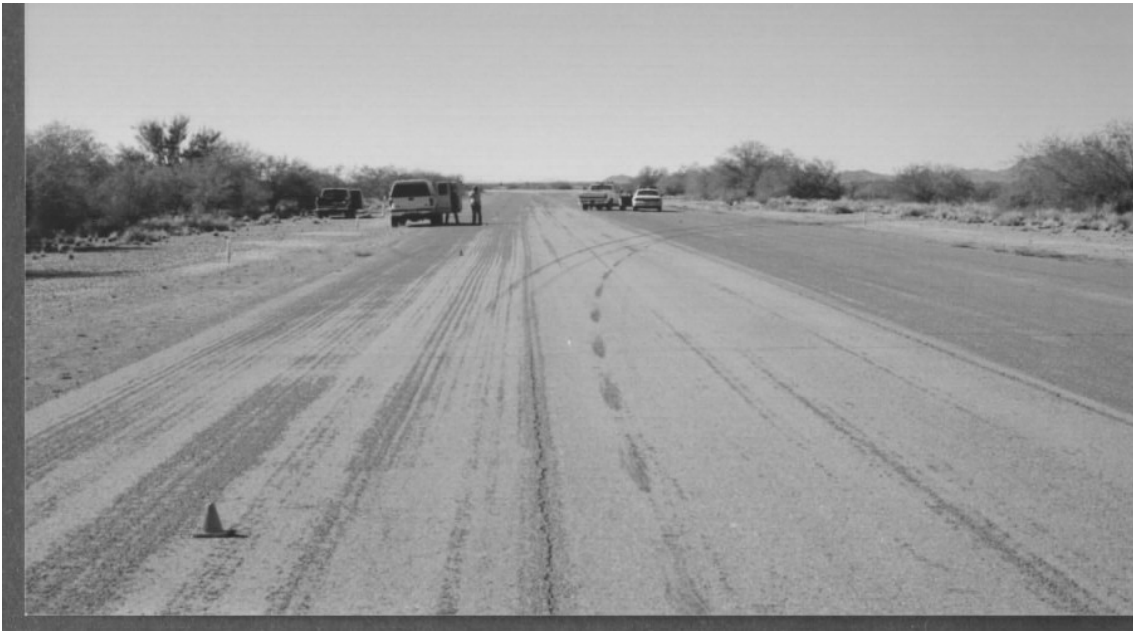
Photograph 2. Hopping rear tire marks
