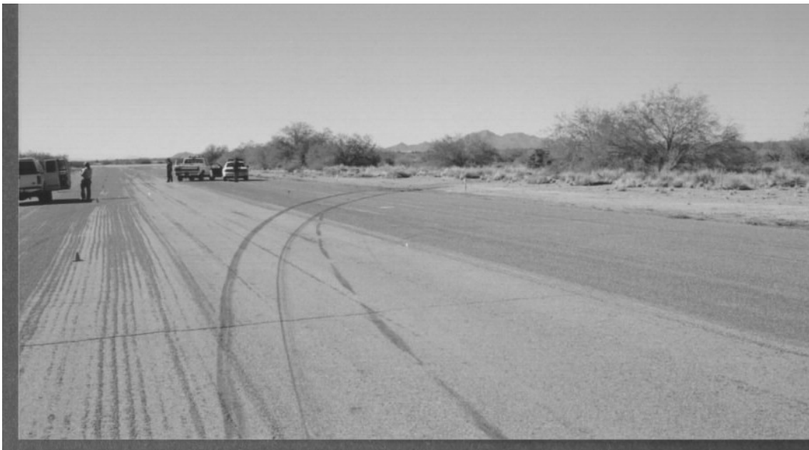
Photograph 4. Hopping/wavy rear tire marks
