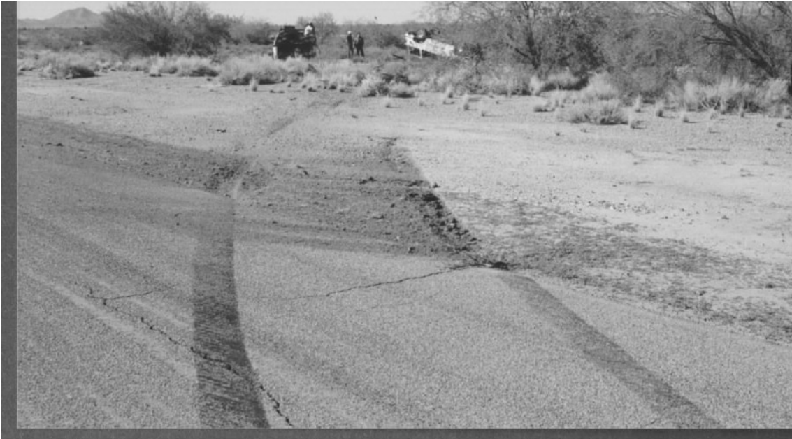
Photograph 5. Left tire marks, hopping not present
