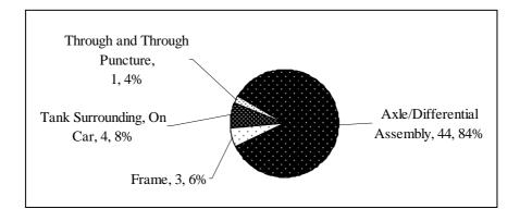
Figure 3, Assembly/Mechanism of (F)ront Failures
