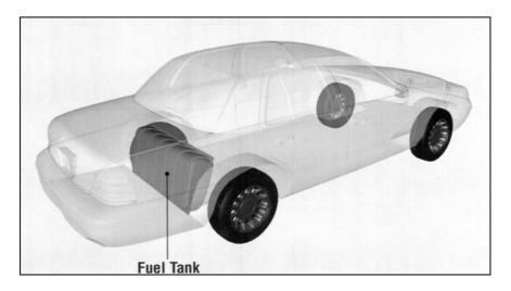
Figure 1, CVPI Vertical-Behind-The-Axle Fuel Tank
