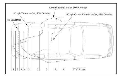
Figure 4, CDC Damage Extent and Typical Crash Test Damage
