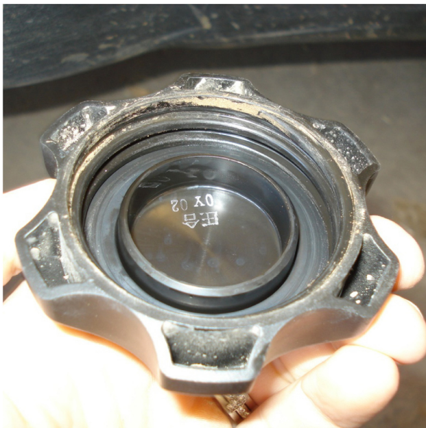
Figure 5. Three of the caps had integral cover, seal and attachment by threads on the outside of the filler pipe.
