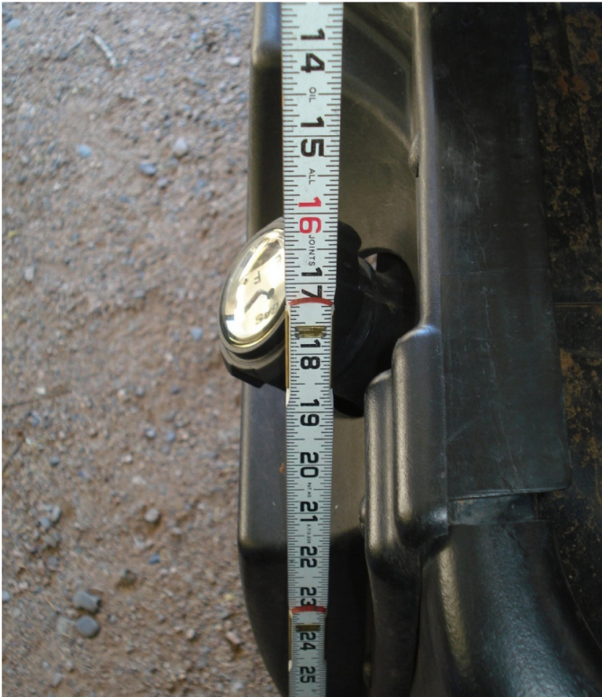
Figure 8. If the vehicle rolled onto its side, interference between the ground and fuel cap would occur.
