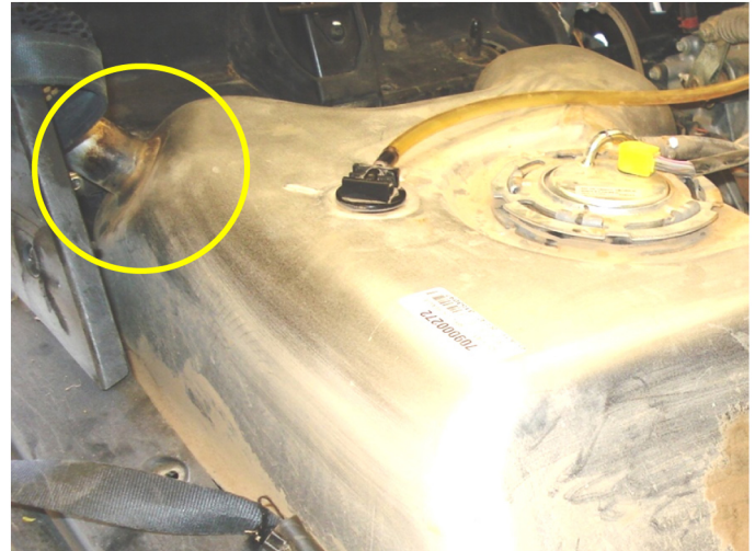
Figure 4. An example of a fill pipe attachment that enters below the top of the tank, preserving vapor space.
