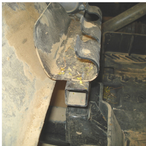
Figure 15. Examples of sharp objects in close proximity to ROV fuel tank.
