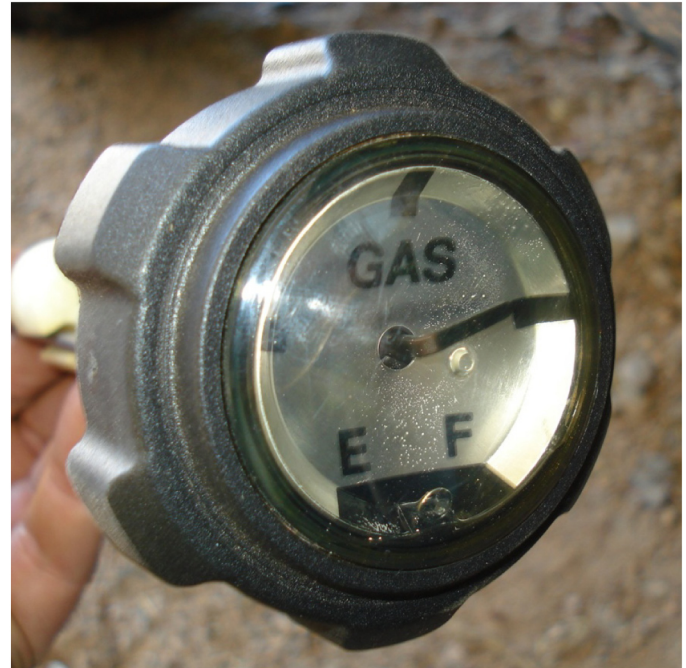
Figure 6. Gauge mechanism allowed gasoline flow through small hole which accumulated between the display and plastic cover.
