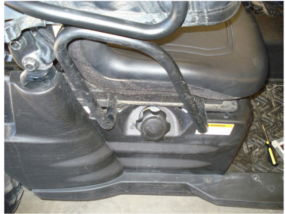
Figure 10. Steel tubes attached to a removable seat appeared to protect a fill pipe and fuel cap that would otherwise be exposed.
