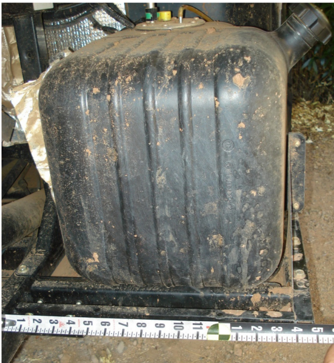
Figure 3. An example of tank location and position relative to structures (covers removed), shown from rear view.
