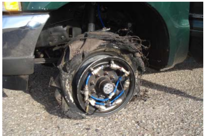
Photo 4. Tire following rapid air-out
