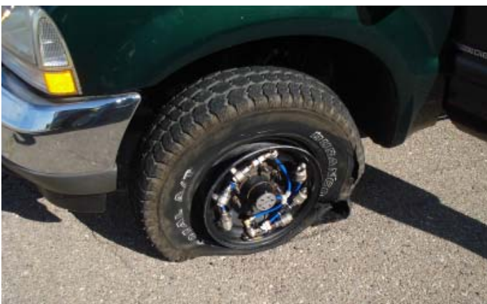
Photo 2. Tire following rapid air-out without tread detachment.
