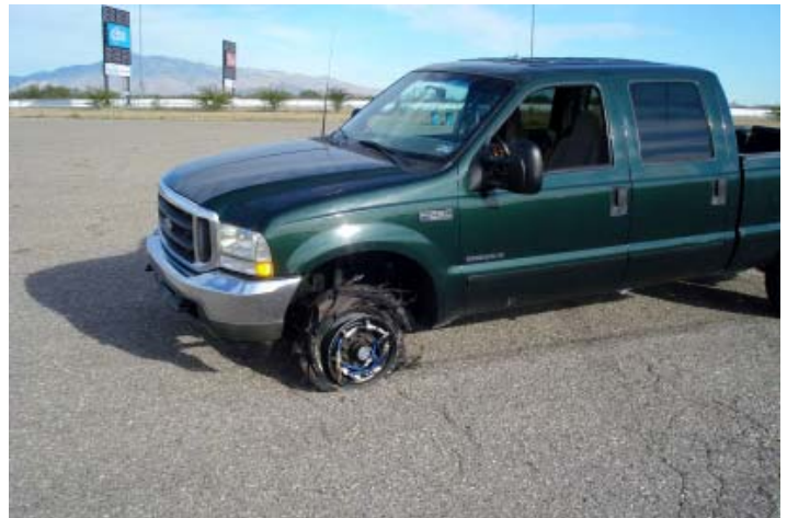
Photo 3. Test truck following rapid air-out with tread detachment.
