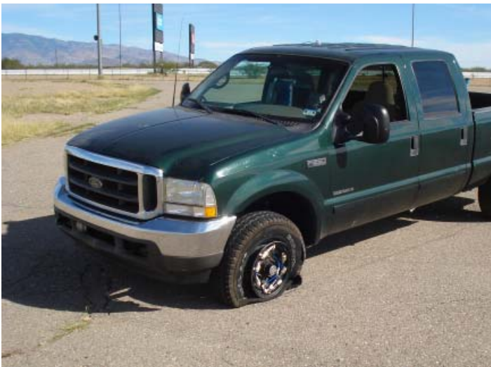
Photo 1. Test truck following rapid air-out without tread detachment.
